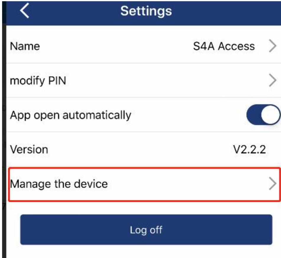
Click manage device, you can rename the reader, adjust the reading range, choose the reader's output format Wiegand 26 or Wiegand 34
