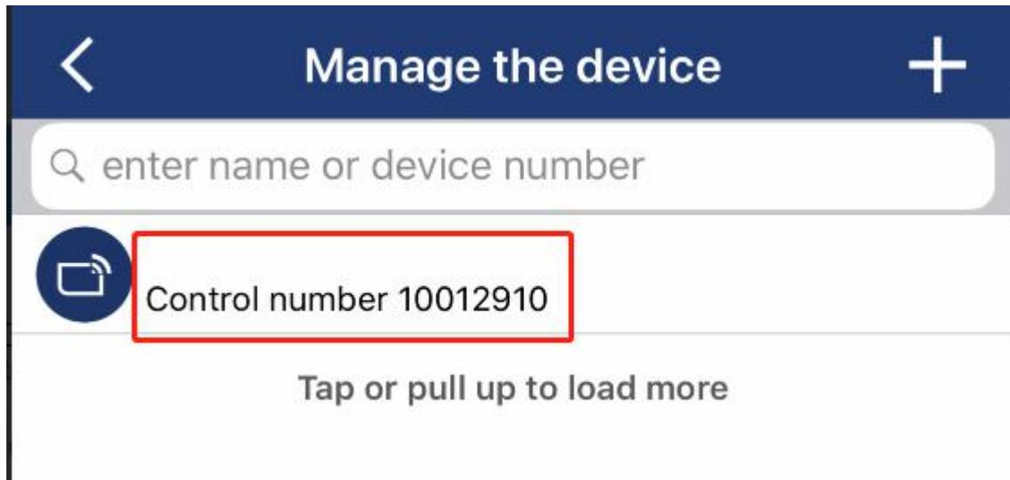
Click the device you want to setting, you can change the device name, adjust the reading range, choose the reader's output format Wiegand 26 or Wiegand 34, photo as below:
