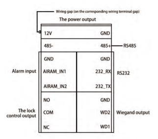
Line gap (under the gap of corresponding terminal)
